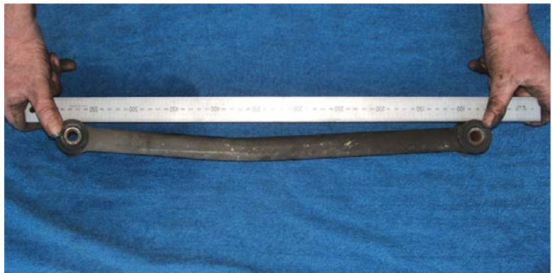
Bent rear suspension lower control arm
