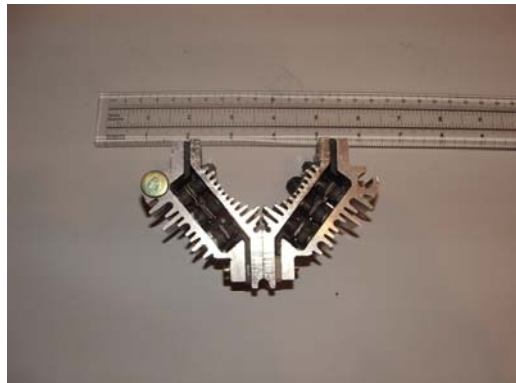
Three phase rectifier, front view
