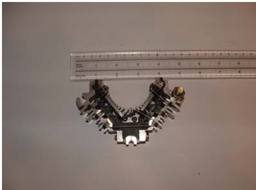
Three phase rectifier, rear view
