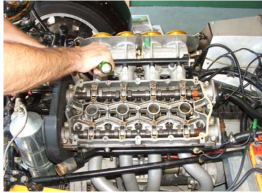
Cam housing and exhaust system installed
