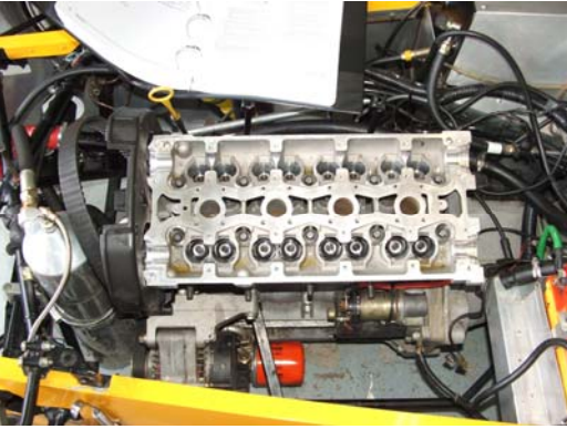
Cylinder head bolt installation
