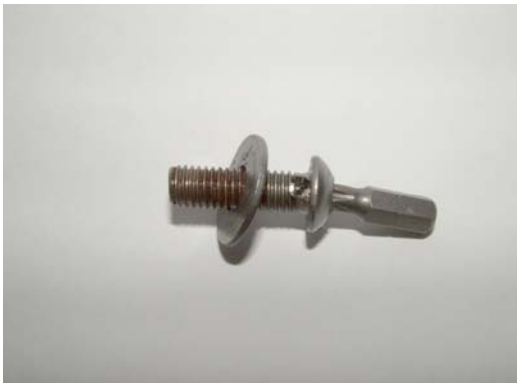
Offending "frozen screw" and driver bit
