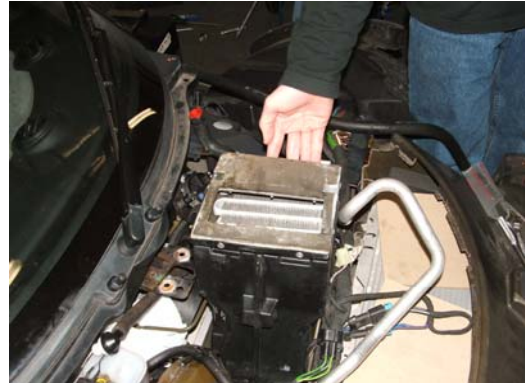
Heater & A/C unit slides upwards to remove
