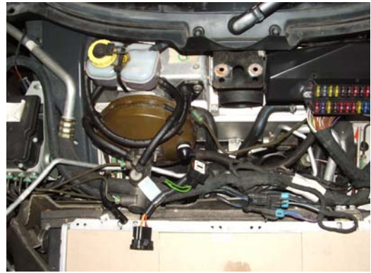
Blower motor unit is located under the brake servo
