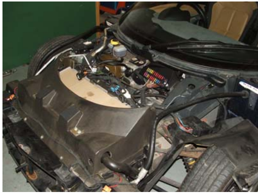
Protective cover installed on top of radiator
