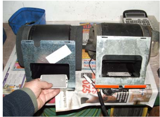
Replacement blower unit is not the same as the original
