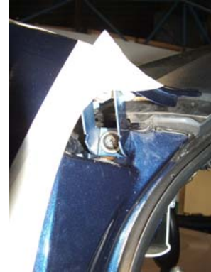
Seized stainless steel fastener at the bottom of passenger side windscreen pillar
