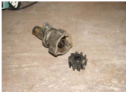
A dismantled charge cooler pump reveals the rubber impellor had failed. This results in a reduction of engine power
