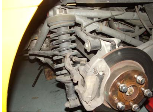
Rear calliper assembled and adjusted incorrectly. Note hand brake lever tight against outer armoured cable.
