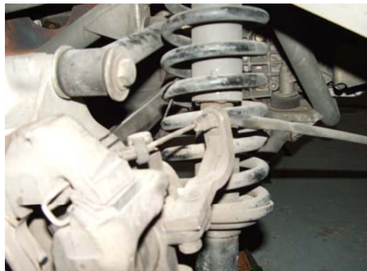
Passenger side rear brake caliper showing the hand brake lever in the correct position
