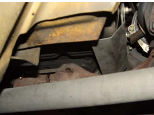
Number 4 cylinder exhaust manifold fastener missing. Note lock tab still in position which was re-used after installing a new fastener
