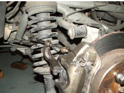
Drivers side rear brake caliper showing the hand brake lever in the correct position after remedial action
