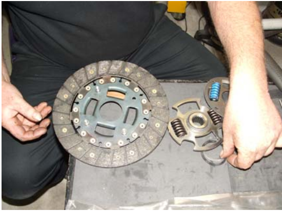
Dismantled clutch plate and spring pack
