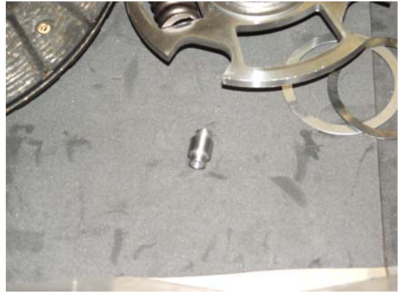
New stepped rivet for clutch plate
