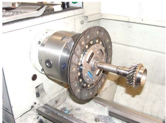
Clutch plate checked for run-out after riveting
