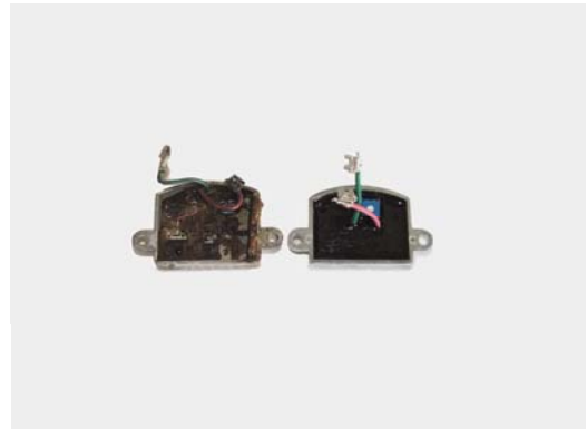
Faulty voltage regulator and replacement
