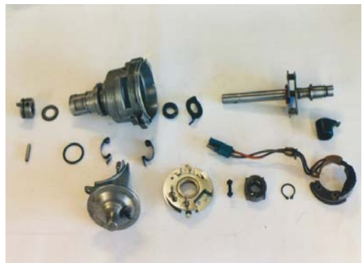
Distributor dismantled to cure invisible oil leak
