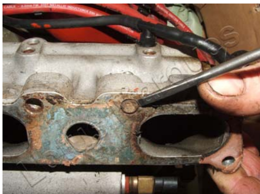
Flip side of broken inlet manifold stud
