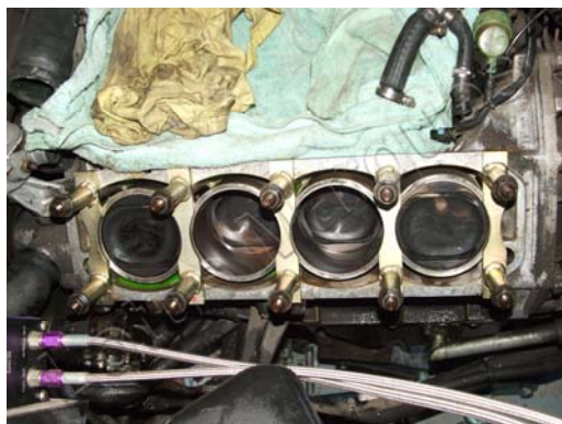
Cylinder head off and liner clamps on Coolant left in engine block for a good reason!
