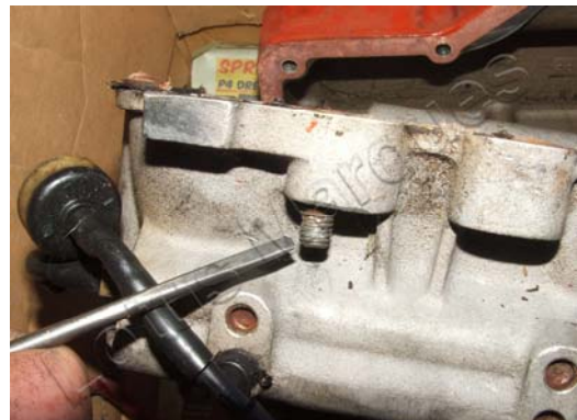
Broken stud retained in manifold
