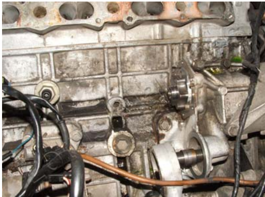
Metal debris inside and outside the engine
