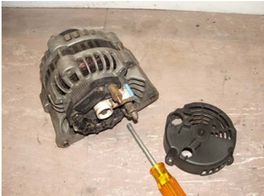
Alternator cover removed
