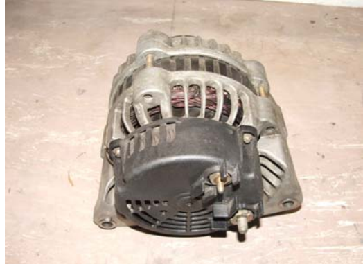
Reinstall plastic cover to complete the job
