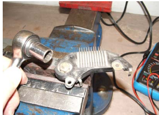
Remove stud from faulty voltage regulator
