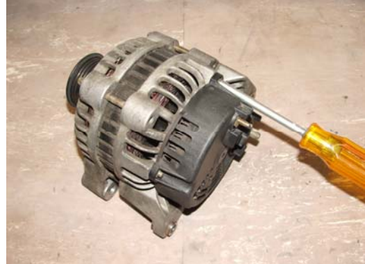
Remove three Torx anti-tamper screws
