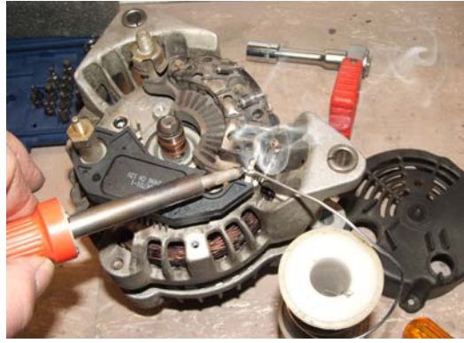
Solder regulator connection
