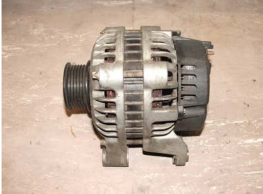
Standard alternator for V8 Esprit
