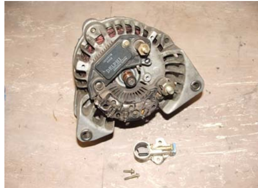
Next, remove brush assembly and check commutator field winding resistance with DVM
