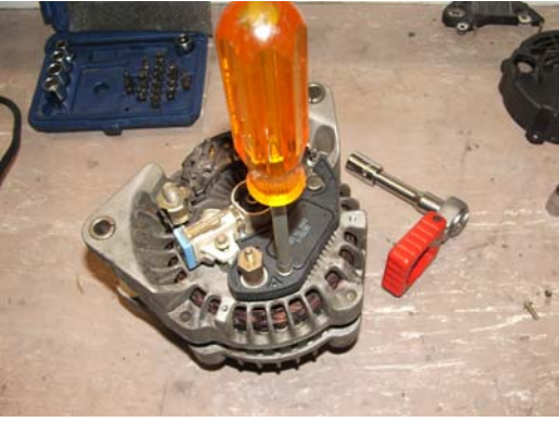
Install new regulator then the brush assembly
