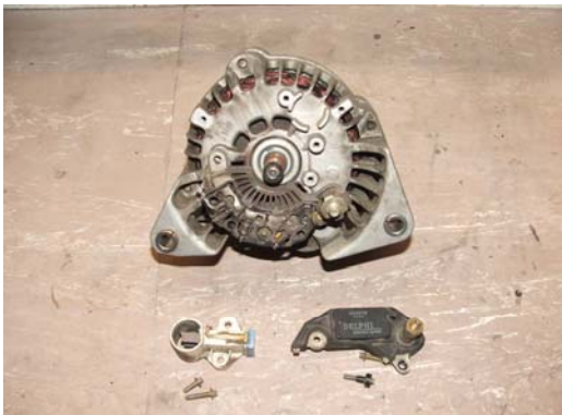
Un-solder, then remove voltage regulator and inspect commutator brushes for wear
