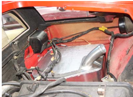
New fuel tank in position
