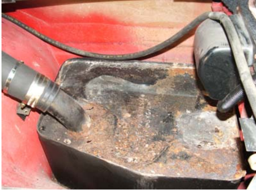
Rusted out fuel tank
