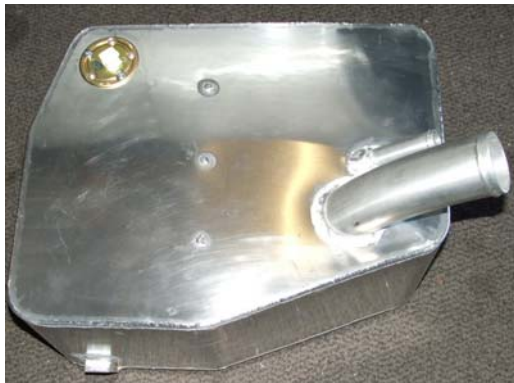
New fuel tank with additional internal baffling
