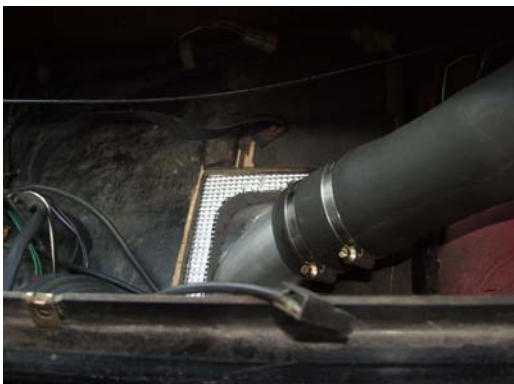
Plywood board secures tank in position
