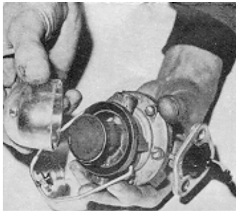
2 Work is easier with the stirrup nut removed. The filter just pulls off - make sure it's free of sediment
