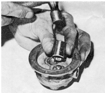
8 Renew seals then fit new valves with suitable hollow drift that bears on outer circumference only
