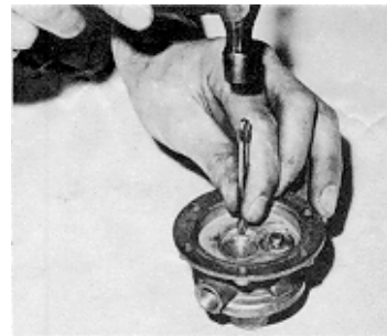
9 The remains of a crosspoint screwdriver was ideal for re-staking, using previous positions as a guide
