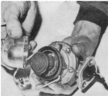
1 Pump off and on the bench, first job was to unscrew the stirrup nut and carefully lift away the glass bowl
